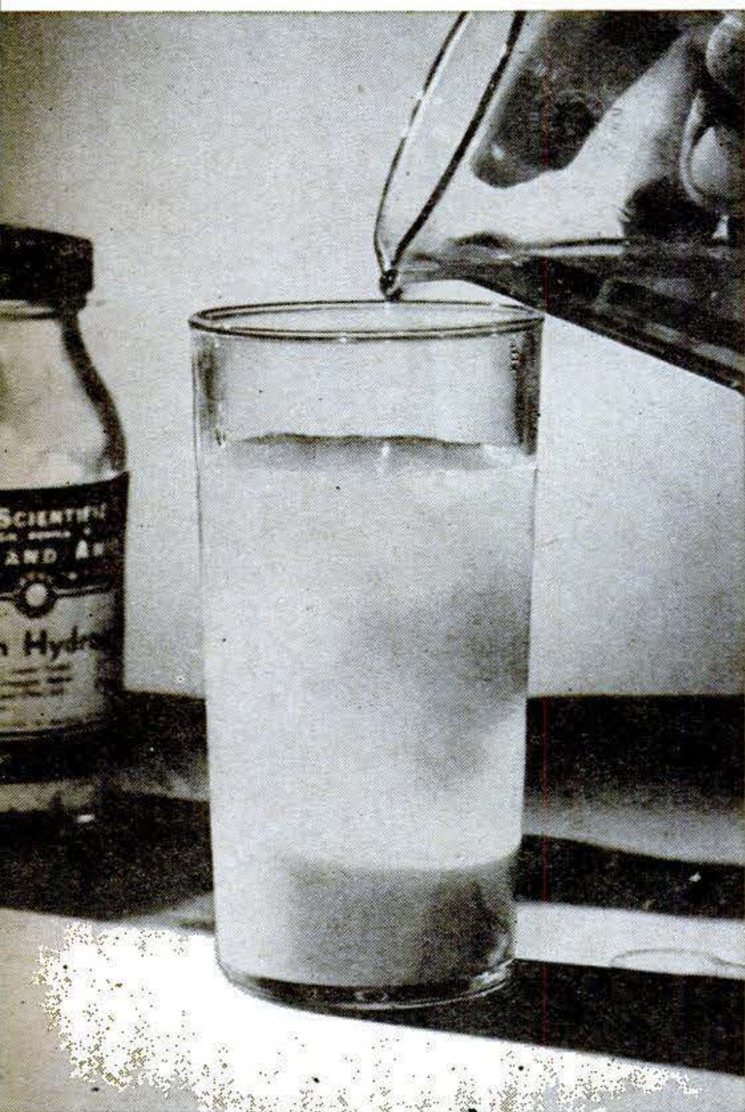
How rayon is made by the cuprammonium process may be shown at home. Add a sodium hydroxide solution to one of copper sulphate.
